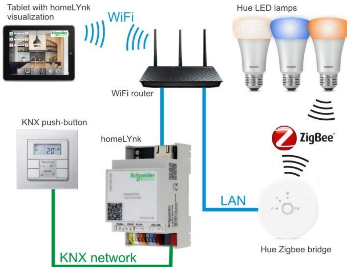
Picture 1: homeLYnk - Philips Hue communication scheme
